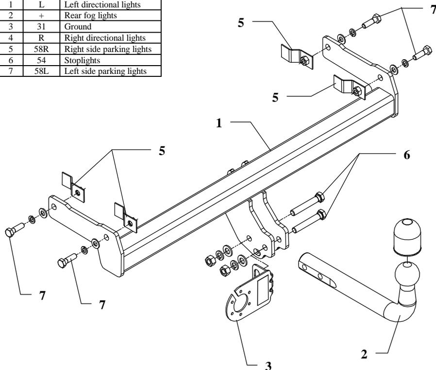
This towbar is designed to assembly in following car: **SKODA FELICIA PICK UP**, produced since 1996, catalogue no. **H11** and is prepared to tow trailers max total weight **1000 kg** and max vertical mass **50 kg**.
